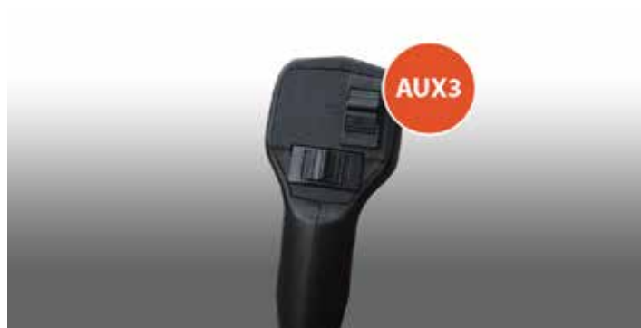
Proportional electronic roller for auxiliary hydraulic system on left Joystick
